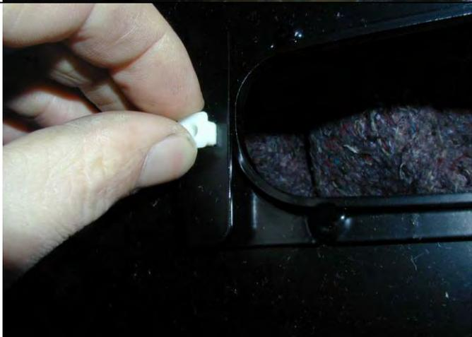
20. Insert nylon nuts into square holes in light brackets inside wing area
