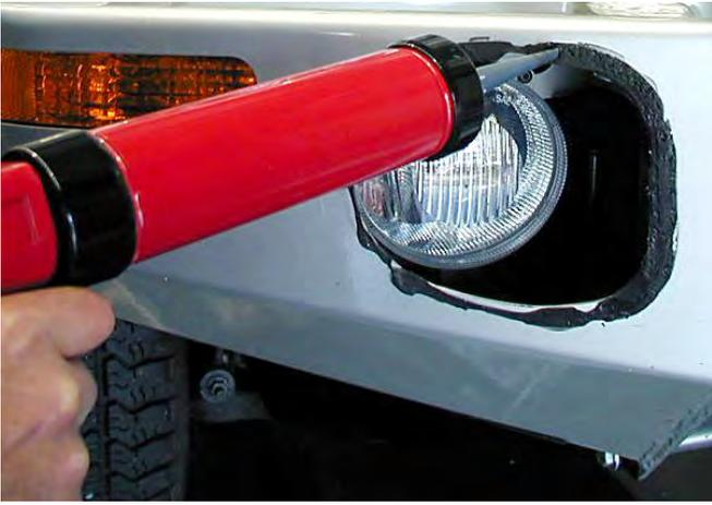
52. Note that the aperture moldings are handed (RH or LH), select correct hand for each wing aperture. Apply Sikaflex to recess in aperture molding flange then fit to aperture in wing. Use adhesive tape to secure plastic mold while Sikaflex cures.
