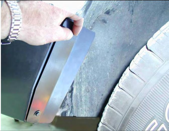
57. Fit liner retainer bracket with black M6 bolt and washer sets into M6 cage nuts in wing returns each side as shown.
