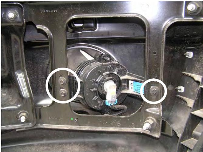
3. If OE fog lights fitted and are required for re-fitment into bull bar, remove each light and bracket assembly and then remove lights as shown by prising the lug each side from the case and undoing the adjuster screw.
