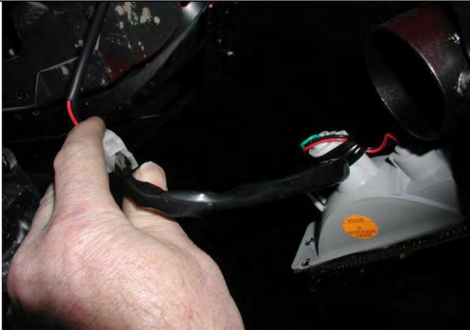
54. Wire up indicators and running lamps. Wire loom extensions are supplied in fitting kit.
