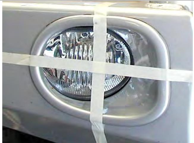
53. Use adhesive tape to secure plastic mold while Sikaflex cures.
