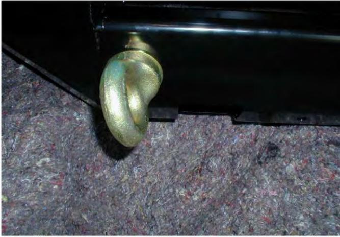
23. Screw in the eyebolt using the large washer. Eyebolt can be positioned to sit vertically by rotating the large nut to the correct position
