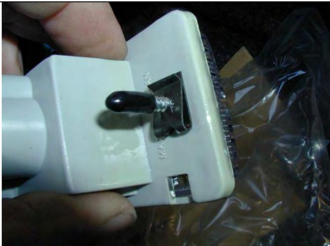
19. Remove lights from cartons and then remove screws and speed nuts from each light. These fasteners are not to be reused – new screws are supplied in the fitting kit
