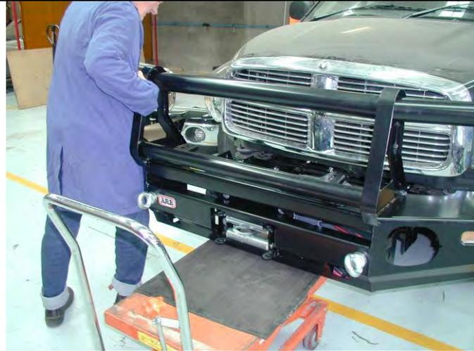
40. Using two people, three if winch fitted, position the bar assembly on the vehicle mounts.
