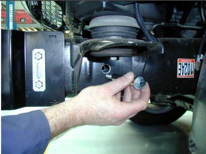
11. As shown, fit M10x100 bolt, sleeve, M10 x 3mm washer and flange nut and do up tight.
