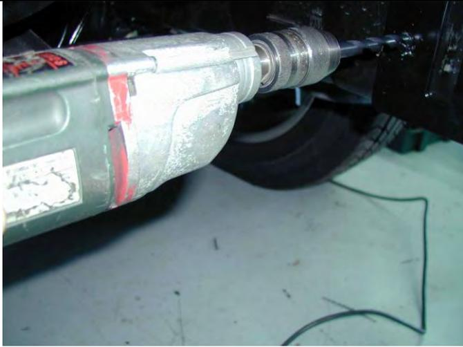
7. Create a starter point with Dia 10.0mm drill using pilot hole in mount bracket for alignment. This will be a guide for Dia 7.0 through hole, which will in turn be used to create a guide hole for Dia 19.0mm hole saw Step 9.
