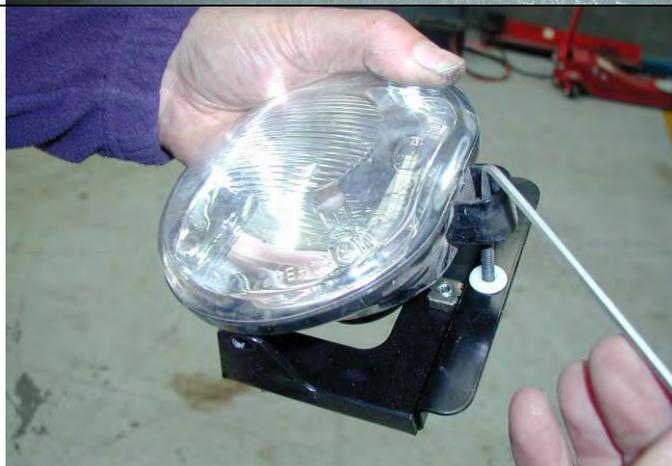
45. Fit light to adaptor bracket by locating mount lugs in light body into holes in adaptor bracket flanges.
