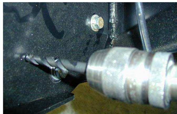
43. Using the M10 pilot holes in mount brackets, drill pinning hole through uprights on bull bar. Fit M10 screw, washer set and flange nut and do up tight.
