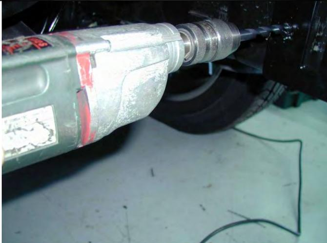
10. Then, as shown, using a Dia 10.0 drill, drill hole through inner wall of chassis.
