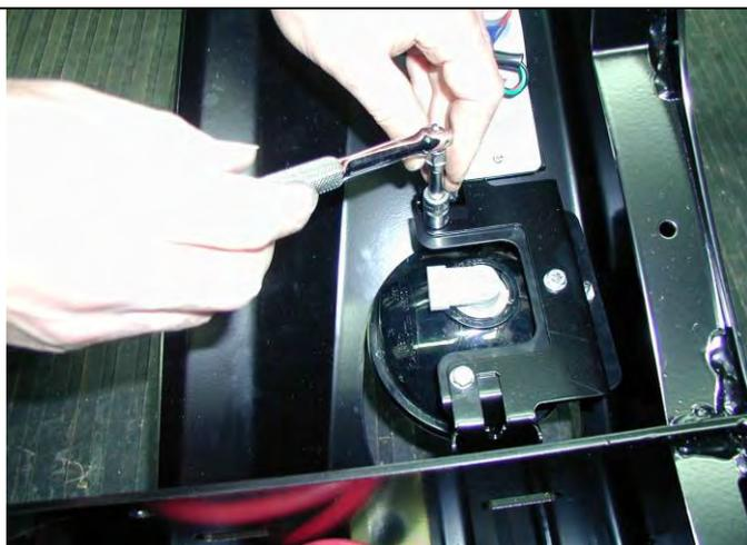
47. Fit adapter bracket and fog lamp assembly into brackets in bull bar wings, as shown.
