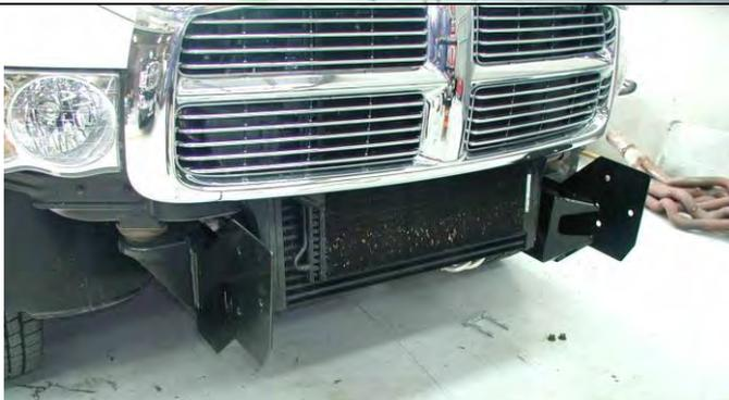
13. Insert original U bolts, entering from **inboard** face of chassis (you may have to tilt intercooler to gain sufficient clearance to allow U bolt to enter this side).
