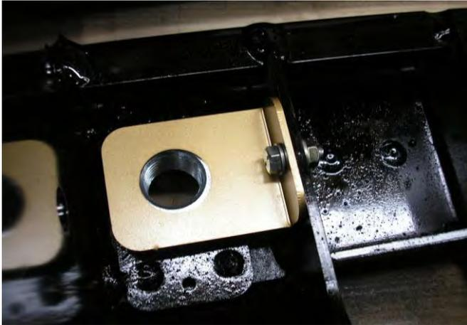
24. When the large nut is in its final position, secure with the nut retaining bracket using an M6 bolt, washer and flange nut.
