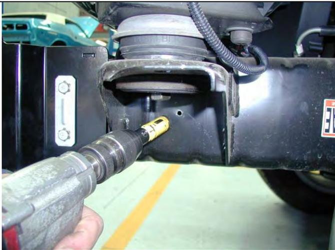
9. Use the Dia 19.0 hole saw, as shown, with 7.0mm hole as a guide to drill a hole through outer wall of chassis.
